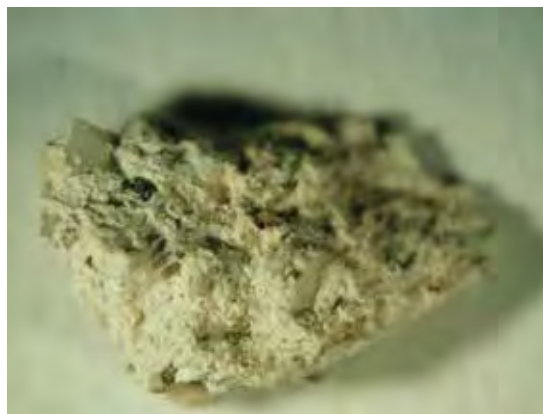
Fig. 57. Stereomicroscope image of the back of paint sample T6 where the supporting plaster made with lime and sand is observed.
