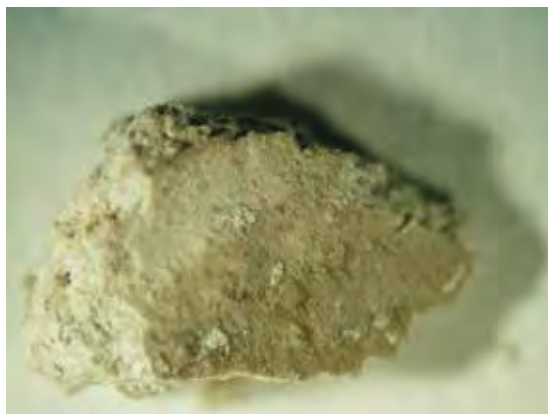
Fig. 56. Stereomicroscope image of the front of paint sample T6 where the white colour of the paint and the presence of surface deposits are observed.
