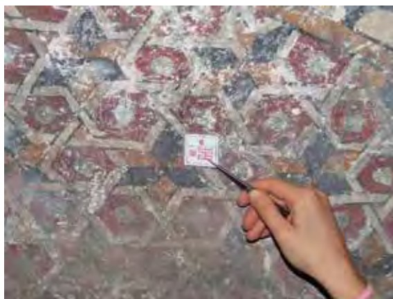
Fig. 55. Sampling point of the microfragment of mural painting T6 with white paint taken from lateral dome 1d - south side - al-Ashrafiyyah.
