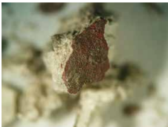
Fig. 7. Stereomicroscope image of the front of paint sample T4 where the red colour of the paint and the presence of surface deposits are observed.
