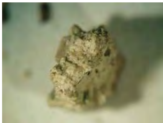
Fig. 8. Stereomicroscope image of the back of mural paint sample T4 where the plaster support made from lime is observed.
