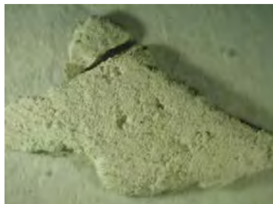
Fig. 24. Stereomicroscope image of the back of paint sample T22a where the white supporting plaster is observed.
