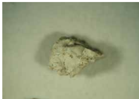
Fig. 46. Stereomicroscope image of the back of paint sample T7 where the supporting plaster made with lime and sand is observed.
