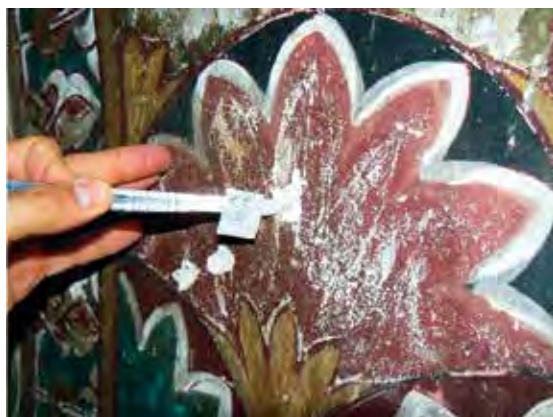
Fig. 14. Sampling point of the microfragment of mural painting CC3 with red paint taken from the central dome - al-Ashrafiya.
