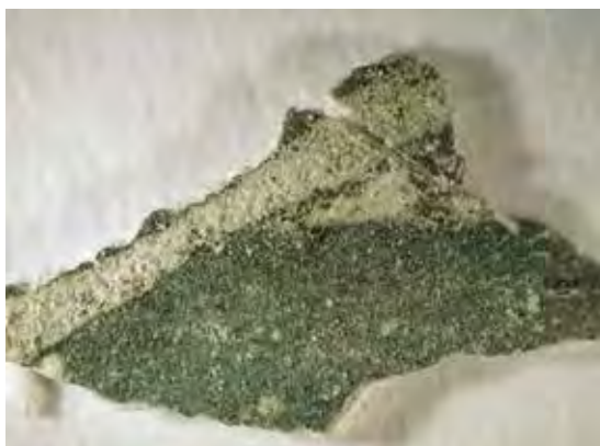
Fig. 23. Stereomicroscope image of the front of paint sample T22a where the blue/green colour of the paint and the presence of surface deposits are observed.
