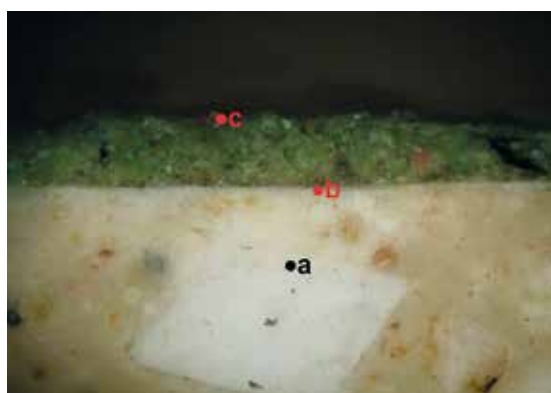
Fig. 47. Image at the optical microscope of the cross section of paint sample T7 viewed in reflected visible light showing the green paint layer (c) containing Green Earth and small quantities of Ochre.
