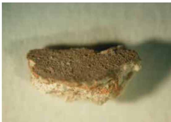
Fig. 37. Stereomicroscope image of the front of paint sample T3 where the yellow colour of the paint and the presence of surface deposits are observed.
